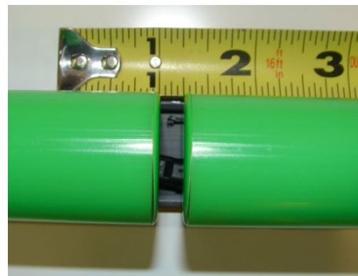
Figure 13 Note: Allow a minimum of a 1/4" Gap between each section for thermal expansion. Failure to leave a gap between sections can cause separation of the product from the mounting surface.
