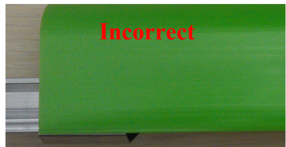
Figure 12: Improperly engaged lens and clip. Note: Lens extends below the top groove, and into the bottom groove of the aluminum channel
