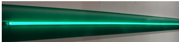
Figure 20: Completed LightBar assembly. Note that no wires are showing, and proper gaps exist between all joints.
