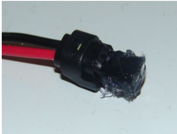
Figure 19: Male plug sealed with silicone. Note the amount used; only use enough to cover the contacts.
