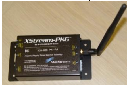
Figure 16: First generation Long Range Radio. (Note: Requires weatherproof enclosure when mounted in a sign.)
