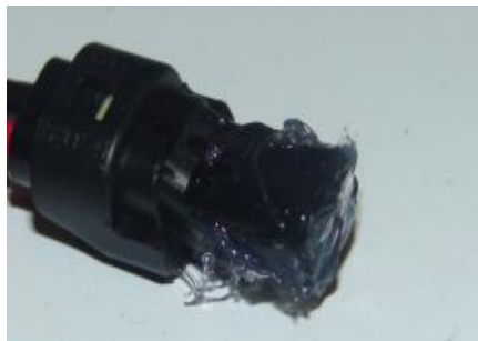
Figure 8: Male plug sealed with silicone. Note the amount used; only use enough to cover the contacts.
