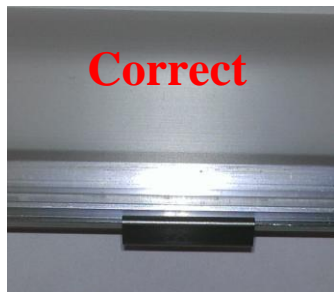
Figure 5: Properly engaged lens and clip. Note: Lens does not extend past the top groove in the aluminum channel
