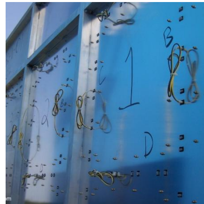
Figure 13: Modular LED digits wiring from behind face
